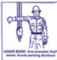
**LOWER BOOM** Arm extended, thumb spread, thumb pointing downward.
