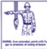
**SWING** Arm extended, palm with finger in direction of swing of boom.
