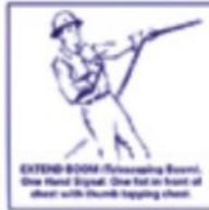
**EXTEND BOOM (Swinging Boom)** One Hand Signal: One fist in front of other with thumb tapping chest.
