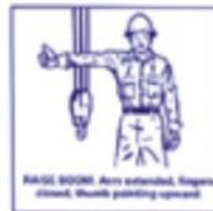
**RAISE BOOM** Arm extended, fingers spread, thumb pointing upward.
