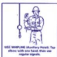
**USE WINDLASS (Auxiliary Hoist)** The elbow with one hand, then use regular signals.
