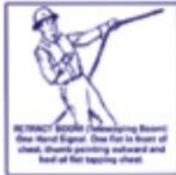
**RETRACT BOOM (Swinging Boom)** One Hand Signal: One fist in front of chest, thumb pointing outward and back of fist tapping chest.
