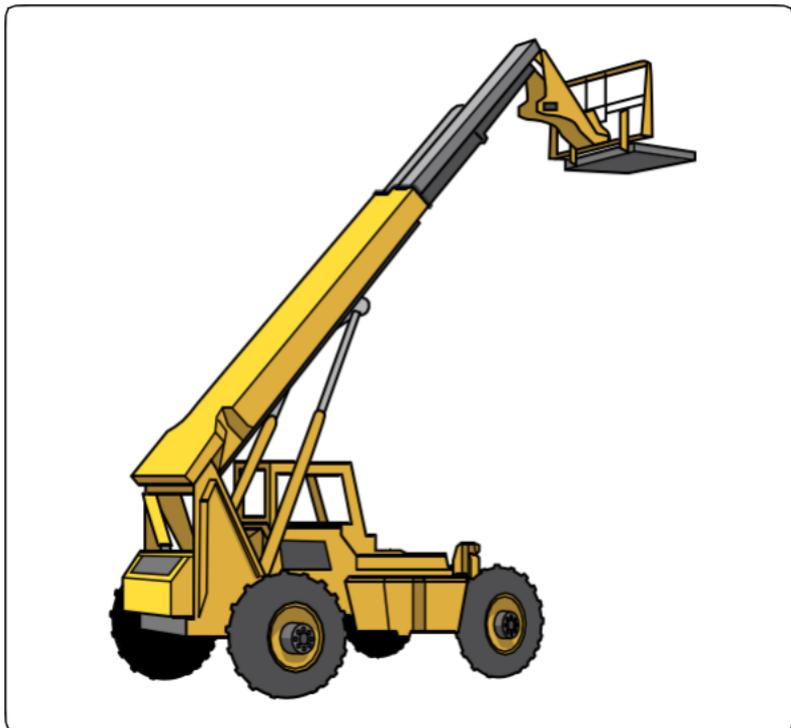
Forklifts and other powered industrial trucks are vehicles such as fork trucks, tractors, platform lift trucks, motorized hand trucks and other specialized industrial trucks that are powered by electric motors or internal combustion engines.
